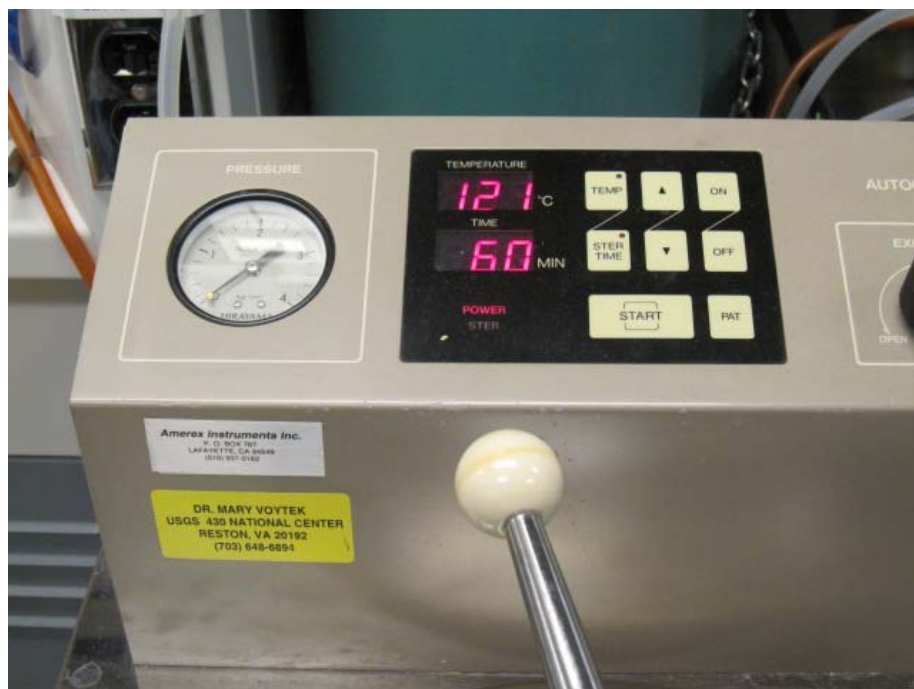
Figure C–2. Autoclaved for 60 minutes at 120 °C.
