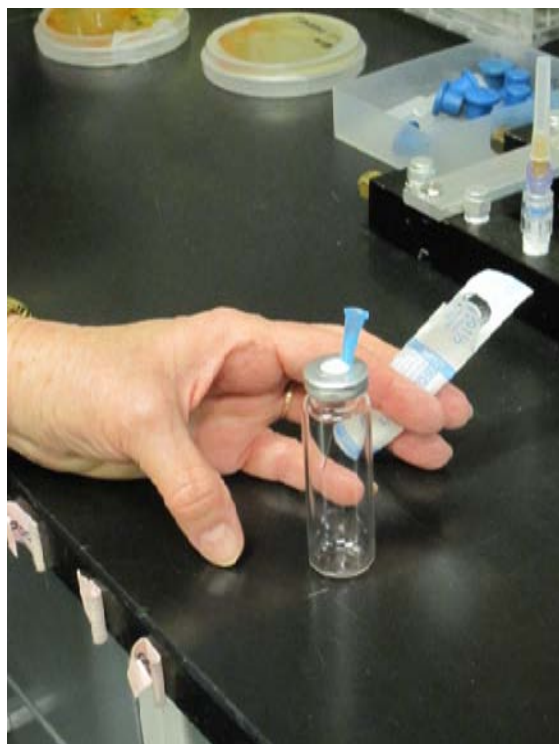
Figure C–14. Empty vial showing placement of vent needle.
