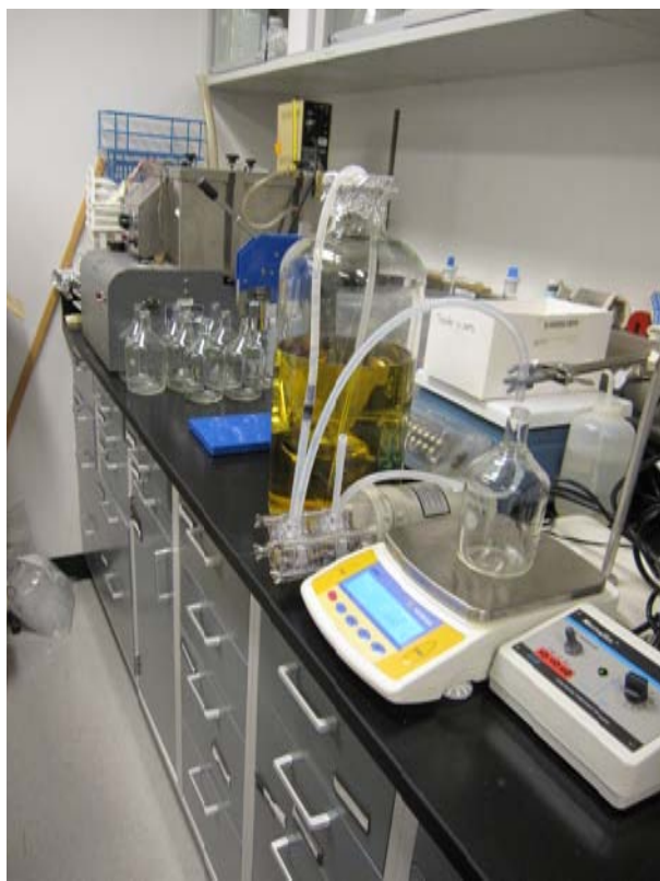
Figure C–1. Tryptic soy broth (TSB), with \text{KNO}_3 , prepared, mixed in 9-L bottle (yellow liquid), and divided into 500-g aliquots.
