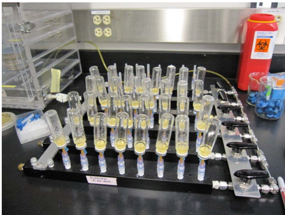
Figure C-15. Manifold showing helium purging of 32 vials.
