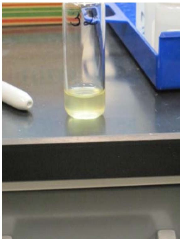
Figure C–11. Twenty-milliliter sample vial containing 3 mL of concentrated cell culture.
