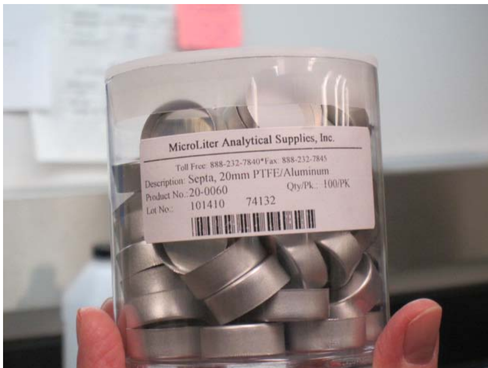
Figure C–13. PTFE/Aluminum-lined septa with aluminum crimps.
