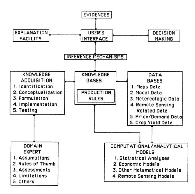
Figure 4.1b. The Architecture of CROPCAST OSU
