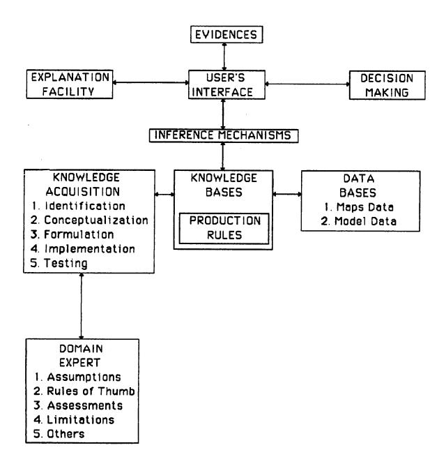
Figure 4.1a. The Architecture of CROPCAST OSU (Phase 1)
