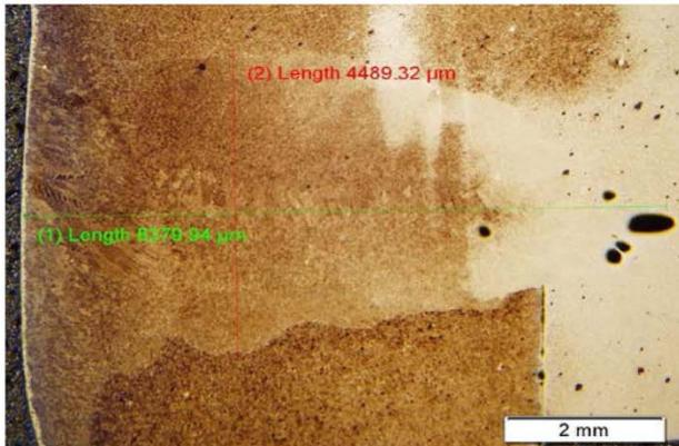
Electron beam weld penetration of > 8 mm with multiple passes
