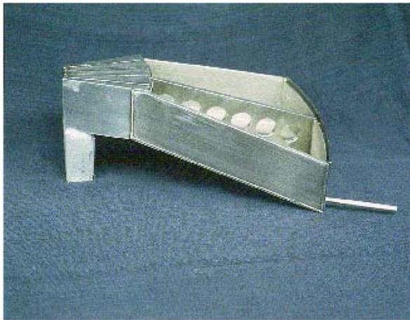
1/10<sup>th</sup> Segment Heat Pipe, Operating Orientation.
