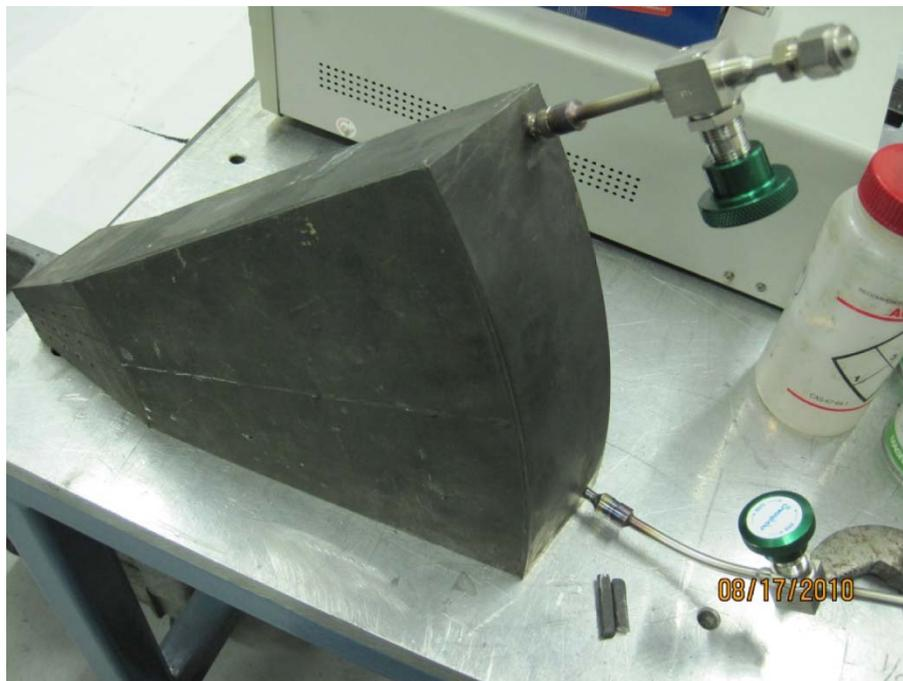
Figure 4.—Vessels attached to heat pipe fill ports.
