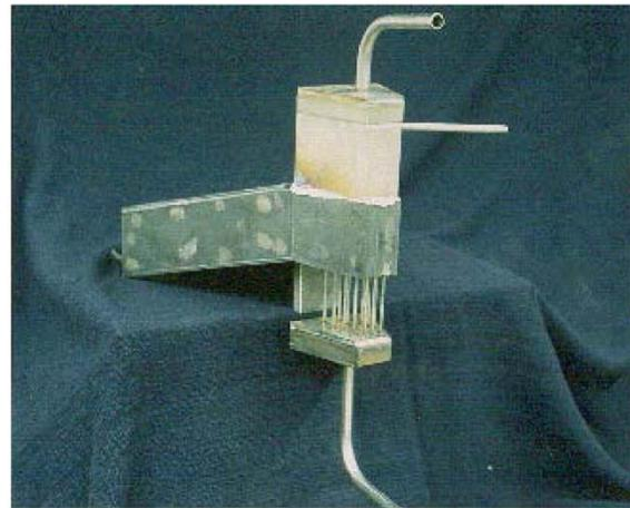
1/10<sup>th</sup> Segment Heat Pipe w/Gas-gap Calorimeter.
