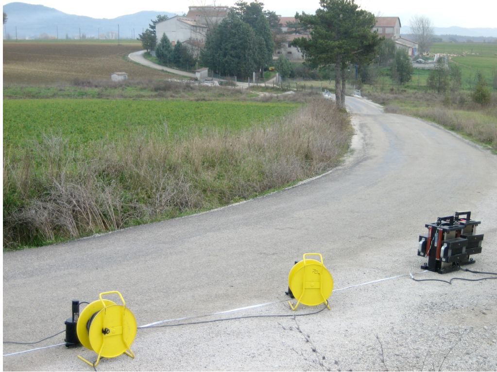
Figure 2. Configuration of the USGS surface wave testing system at site 262GBP Gubbio Piana Soil Site (43.314°N,12.59°E) composed of 1-Hz vertical motion sensors and two-100 kg electro-mechanical harmonic wave shakers. The shaker apparatus are arrayed in a parallel circuit and synchronized in phase.
