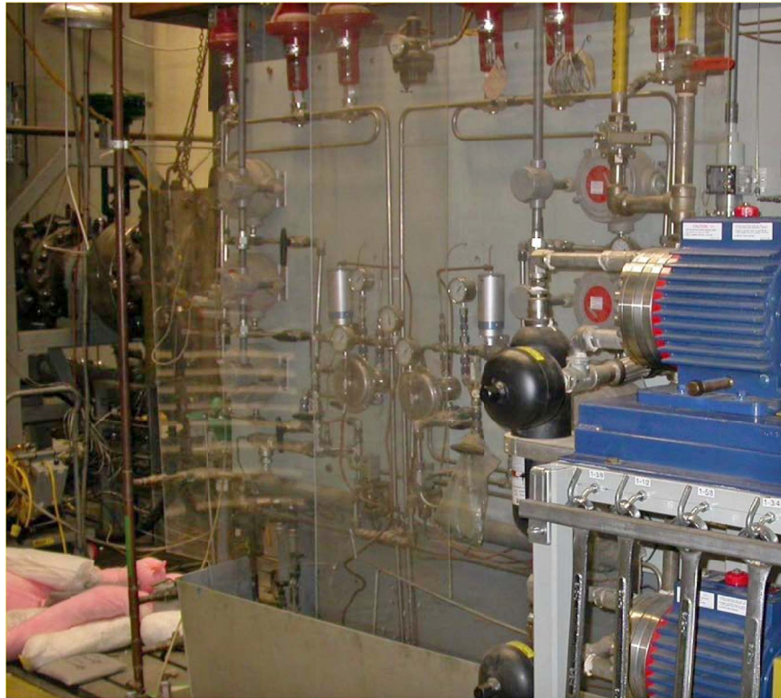
Figure B-2.—Fueling station adjacent to the test section, providing blended fueling on demand. Foreground is the main fuel pump and the secondary blending system in background.
