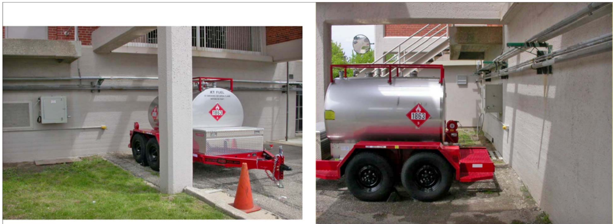
Figure B-3.—Photos of portable alternate fueling transport and facility supply tank.
