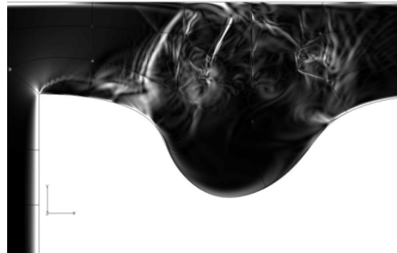
Figure 20.—Density gradient contours in a supersonic tip recess.
