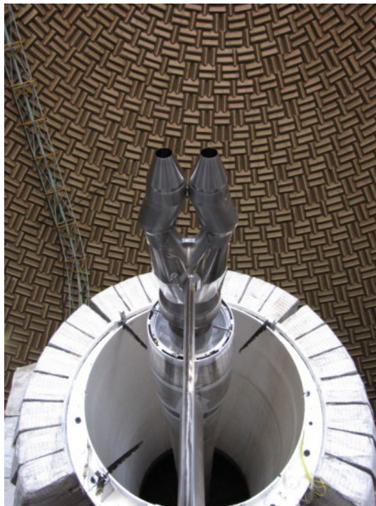
Figure 3.—Twin jet model installed on the High Flow Jet Exit Rig (HFJER) in the Nozzle Acoustic Test Rig (NATR) in the Aeroacoustic Propulsion Laboratory (AAPL) at NASA Glenn Research Center.
