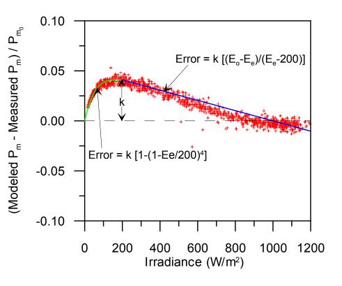
Error in watts normalized by P<sub>mo</sub>
