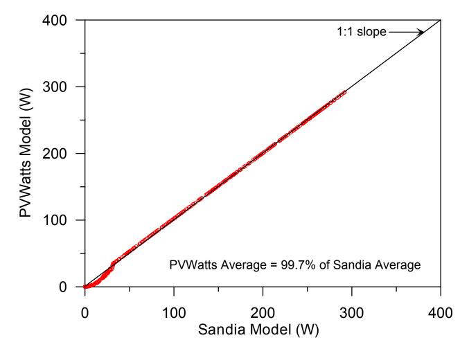
Differences at low irradiances from PVWatts using a different algorithm below 125 W/m<sup>2</sup>.
