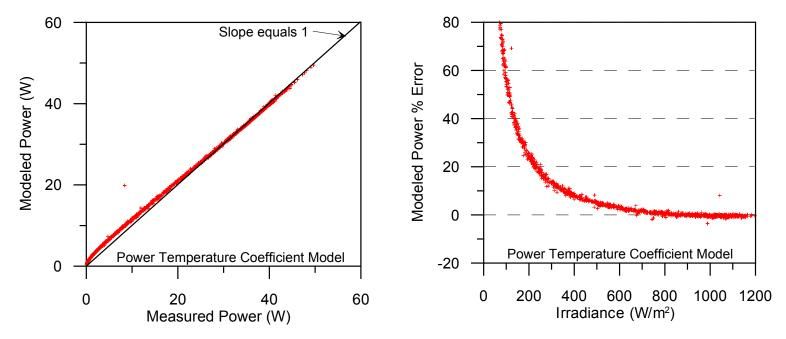
Scatter plot and percent error graph showing nonlinearity with respect to Irradiance for a multi-crystalline PV module.
