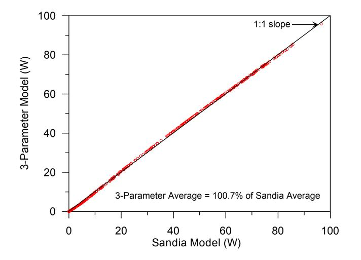
The historical PV model in PVWatts is acceptable for estimating the energy production of PV systems.
