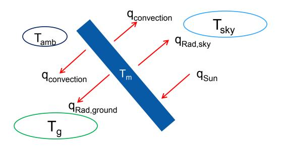
$$\alpha_s G_s = \varepsilon_g \sigma \left(T_m^4 - T_{sky}^4\right) + 2 \left(1.2 * W_{avg} + 4.8\right) \left(T_m - T_{amb}\right) + \varepsilon_b \sigma \left(T_m^4 - T_g^4\right)$$
