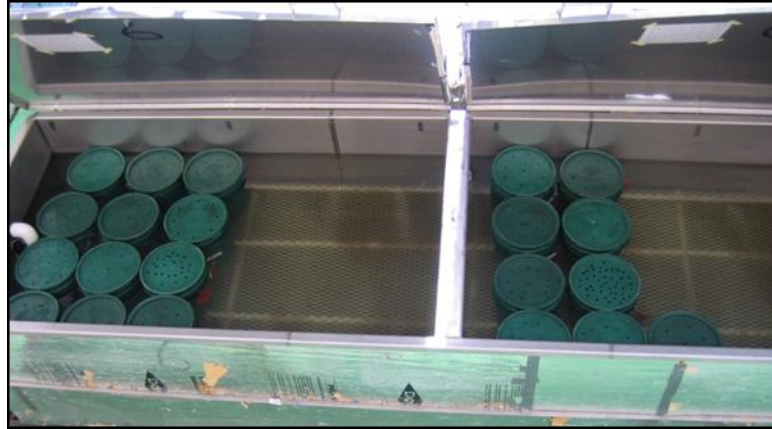
Figure 5. Holding tank with immersed 19-liter perforated recovery containers. The perforations allow water exchange between the containers and the larger volume of the tank.
