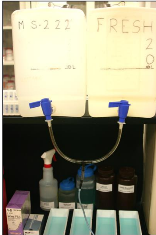
Figure 3. An example gravity feed irrigation system. One container holds fresh water and one container holds a light dose (sedation) of MS-222®. Both containers have valves to control flow. The tubing from each container is joined, and a single line of tubing continues to the surgery platform.
