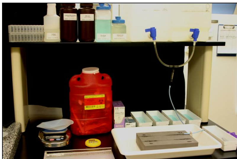
Figure 4. An example tagging station with gravity feed irrigation system, instrument disinfection and rinse trays, and surgical platform.
