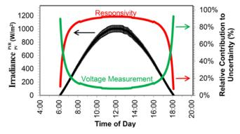
Fig. 1. Calculated POA irradiance for the pyranometer, along with accompanying expanded uncertainty error bars (left axis), and relative contributions to total uncertainty from the inputs to Eq. (2), V and R (right axis).
