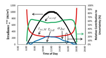
Fig. 2. Calculated POA irradiance for PV reference device, along with accompanying expanded uncertainty error bars (left axis), and relative contributions to total uncertainty from the inputs to Eq. (4).
