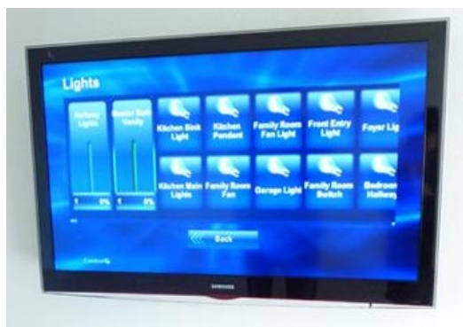
Figure 17. Control4 lighting control interface through the television
