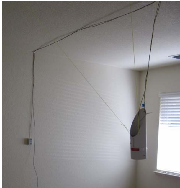
Figure 58. Thermocouples for interior temperature measurements
