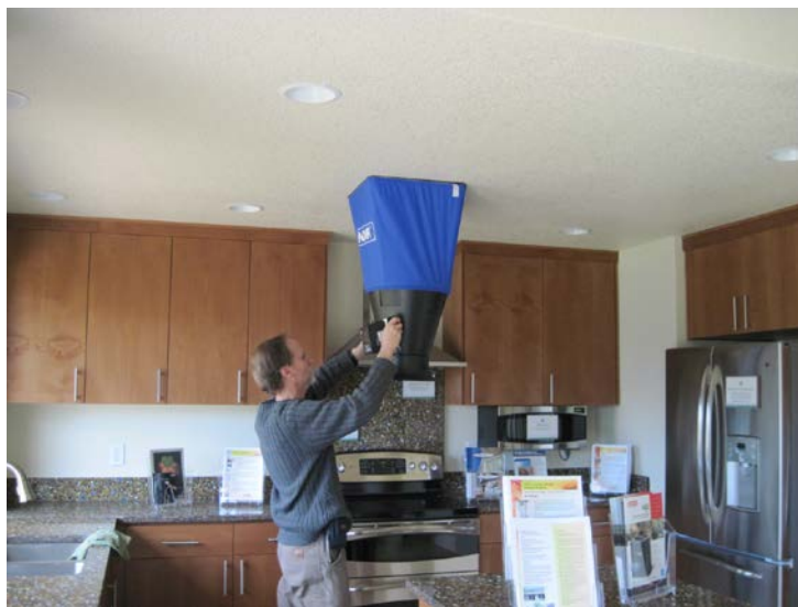
Figure 9. Flow hood test in progress
