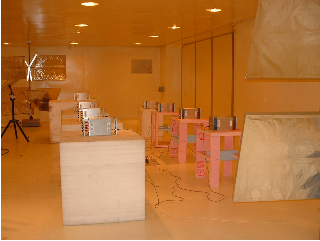
Figure 3: Nodes in chamber A with the shielding enclosures open (optical fibers not shown)
