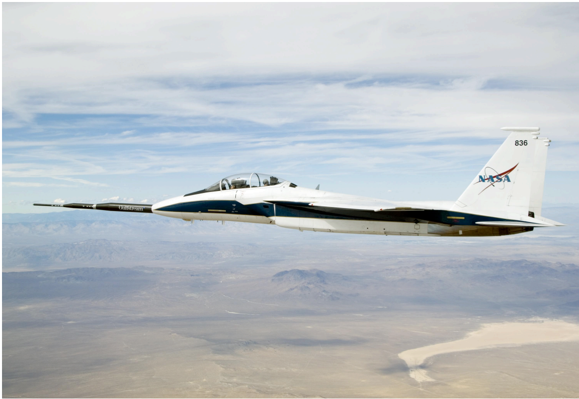
Figure 1. The NASA Dryden Flight Research Center F-15B testbed airplane with the Quiet Spike™ nose boom attached.
