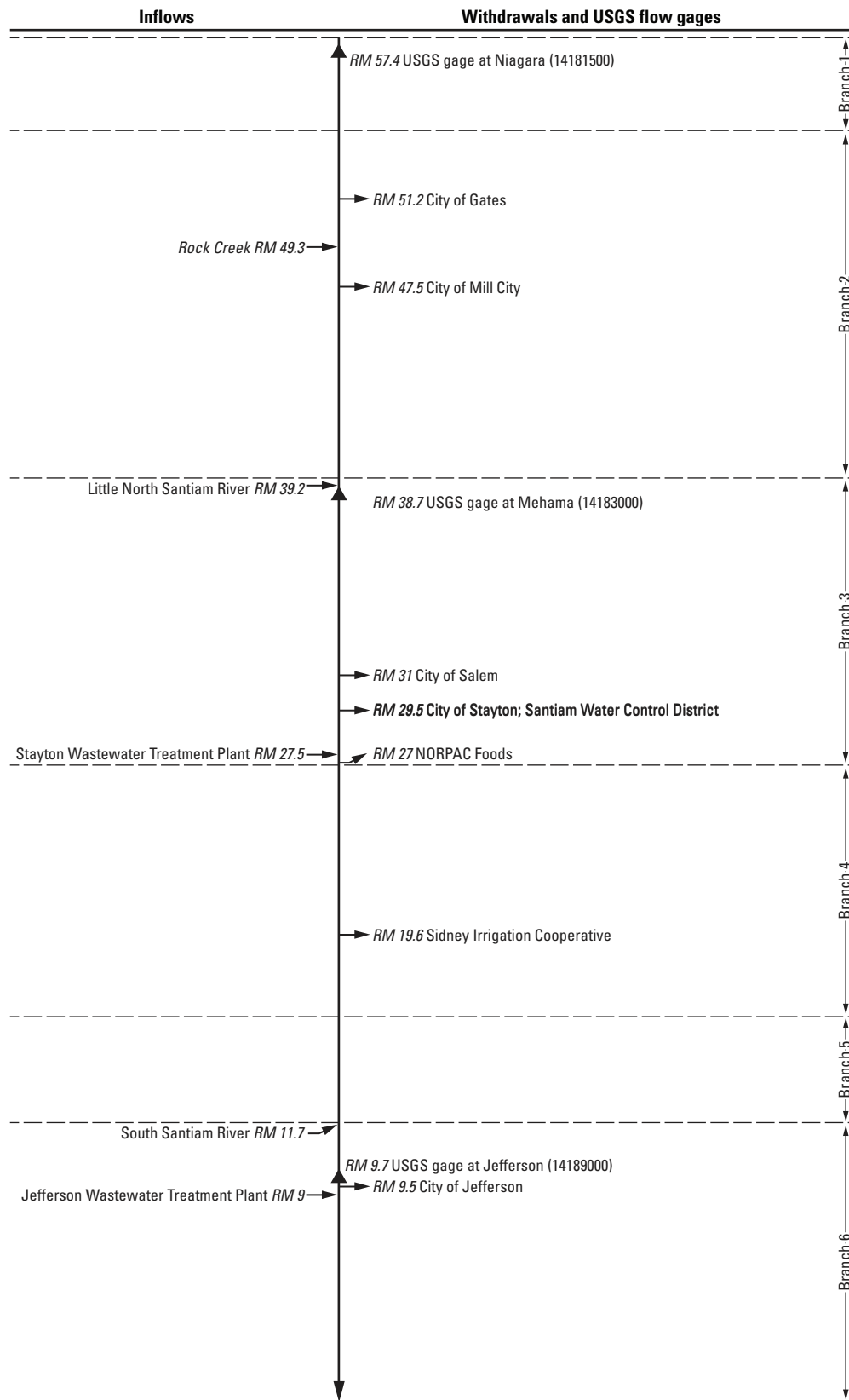
Figure 3. Locations of point-source and tributary inflows, withdrawals, and USGS streamflow-gaging stations in the North Santiam and Santiam Rivers downstream of Big Cliff Dam, Oregon. (Diagram reproduced from Sullivan and Rounds, 2004.)
