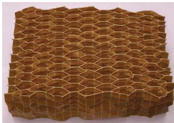
Figure 18. Post-test photograph of the 104-cell DEA component.
