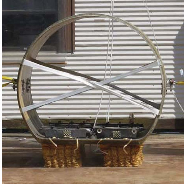
Figure 27. Post-test photograph illustrating DEA crush response.
