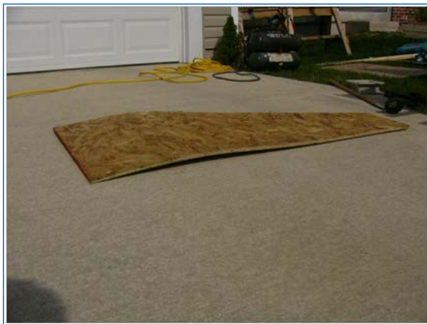
Figure 3. Removed buckled OSB panel
