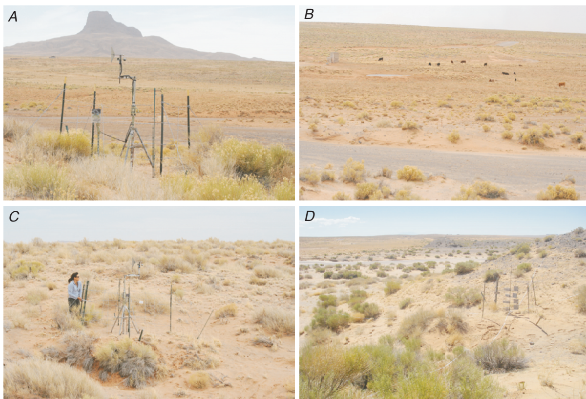
Figure 4. Weather station, sand traps, and vicinity of study site 7 (see fig. 1C for location). A , Weather station, with anemometer and wind-direction sensor mounted on instrument tripod 2 m above ground. The rain gage is on the left; fenced enclosure surrounds the station. View is southeastward across Teesto Wash. B , Cistern and cattle near study site 8, viewed from study site 7 across Teesto Wash. C , Weather station at study site 7. View northeastward. D , Sand-trap deployment at study site 7. Four Big Spring Number Eight (BSNE) sand traps were mounted on a vertical pole and surrounded by a fenced enclosure. White measuring tape along ground was used to measure gap length during ground-cover surveys. View southwestward.
