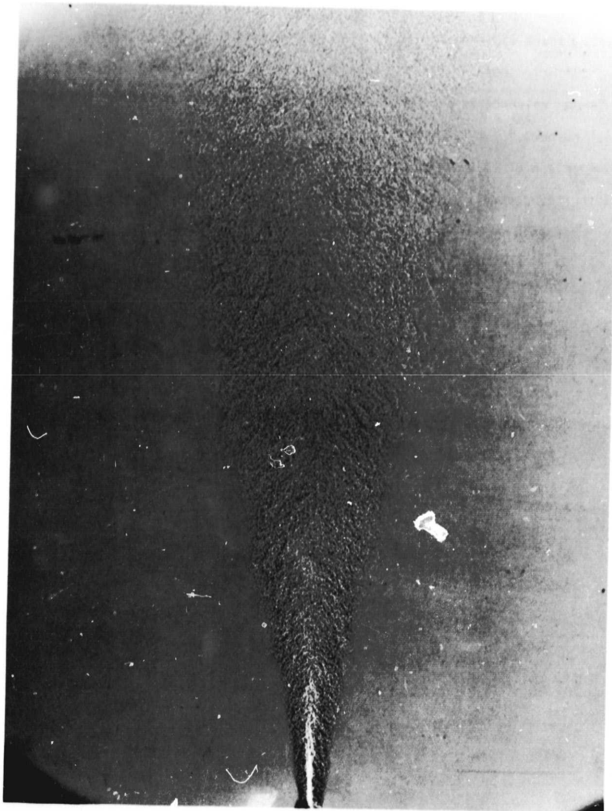
Figure 16. Shadowgraph flow picture of the free-jet. M_{ex} = 0.25 .
