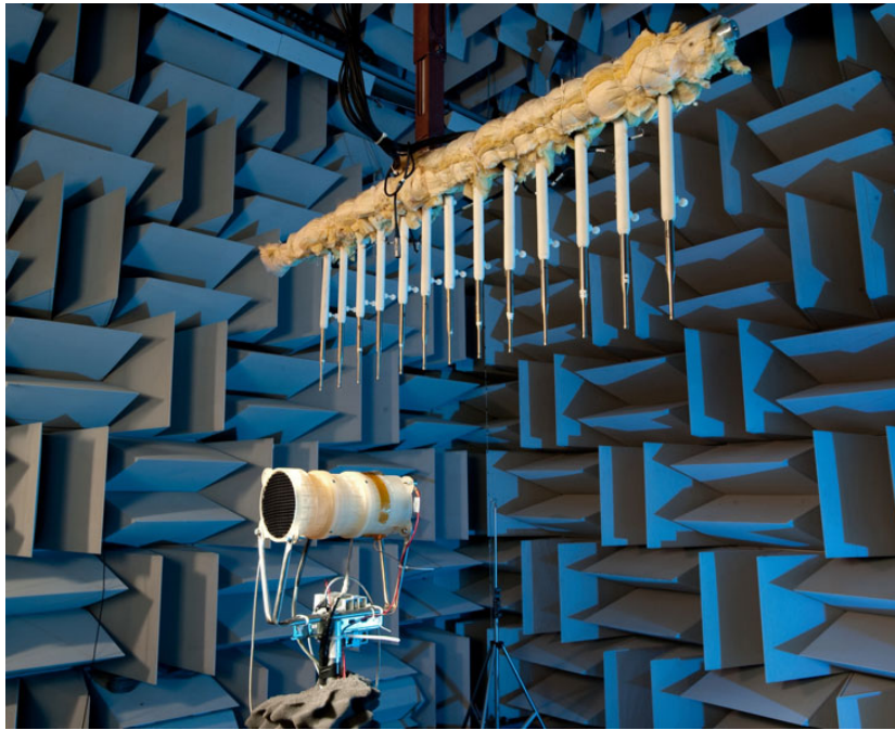
Figure 8.—Photograph of spacecraft cabin ventilation fan prototype and traversing microphone array in the NASA Glenn Acoustical Testing Laboratory
