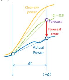
Figure 5. Graphical representation of short-term forecast for solar
