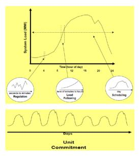
Figure 1 Power system time scales
