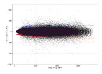
Figure 2. Wind 10-min forecast errors versus power output, along with 95% confidence interval bands
