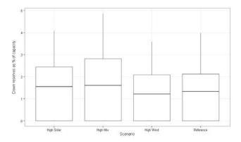
Figure 11. Distribution of flexibility down reserves relative to installed capacity for the WI
