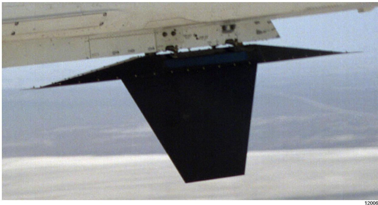
Figure 3. The NASA F-15B testbed aircraft with the Supersonic Natural Laminar Flow test article.
