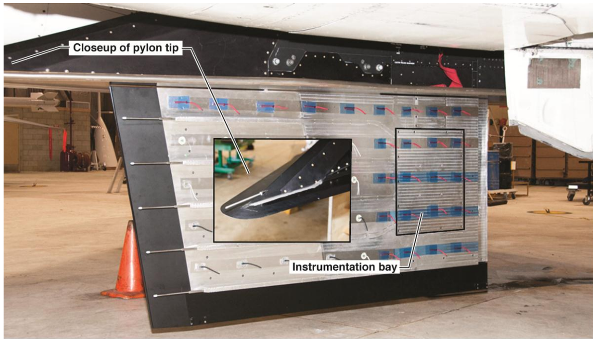
(a) Test fixture backside, showing the strongback and local flow measuring probes.
