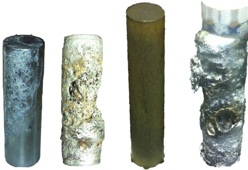
Figure 8. W-Re-HfN samples, before testing and after failure.
