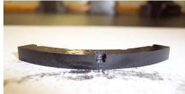
Seal Ring wear during test phase of advanced design misalignment tests
