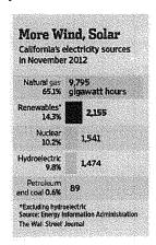
California has encouraged growth in solar and wind power to help reduce greenhouse-gas emissions. At the same time, the state is running low on conventional plants, such as those fueled by natural gas, that can adjust their output to keep the electric system stable. The amount of electricity being put on the grid must precisely match the amount being consumed or voltages sag, which could result in rolling blackouts.
