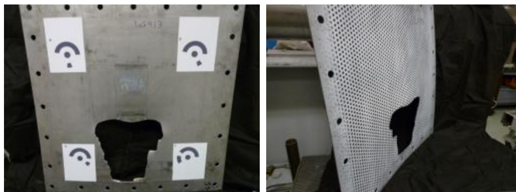
Figure 37.—Large Ti-6Al-4V Test Panel, front and back side, test LG913.
