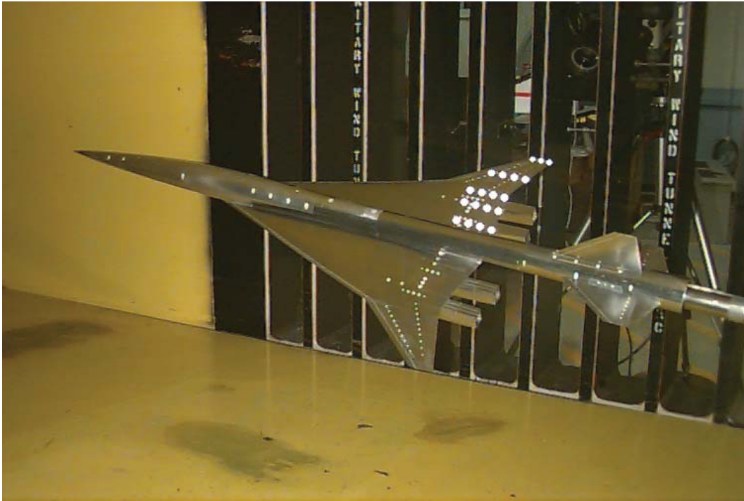
Figure 1. Supersonic transport airplane model with retroreflective targets on right wing upper surface for video model deformation testing in the NASA LaRC UPWT.
