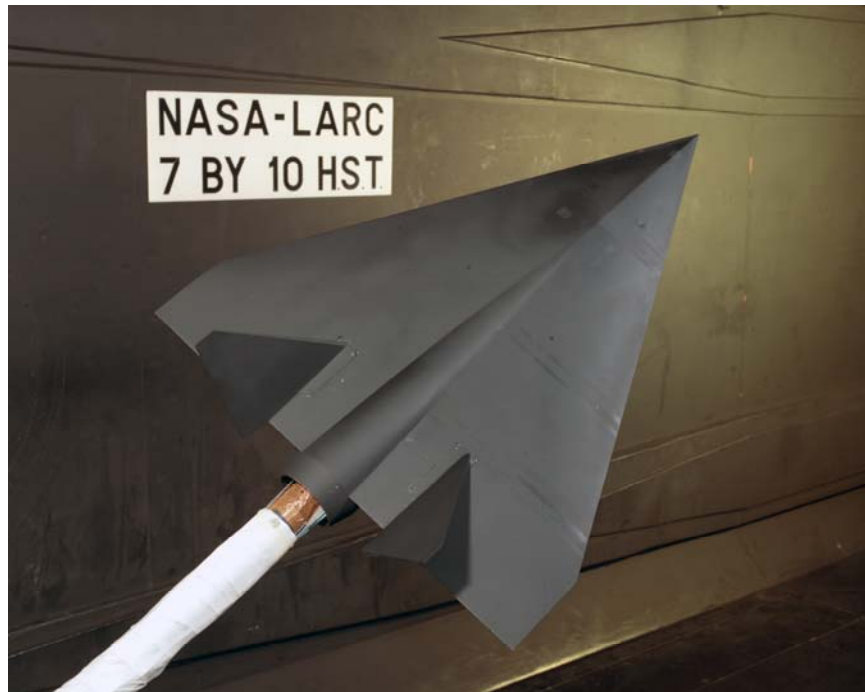
(c) 65° cropped delta wing model with twin canted tails; LEX off
