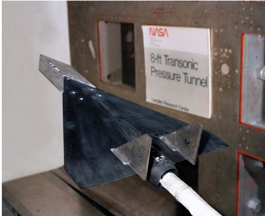
(b) Porous LEX-wing configuration with twin uncanted tails
