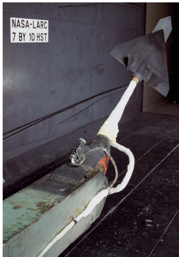
(a) high angle-of-attack static stability support system
