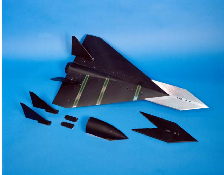
Figure 1. Several of the key components of the 65-degree cropped delta wing wind tunnel model.
