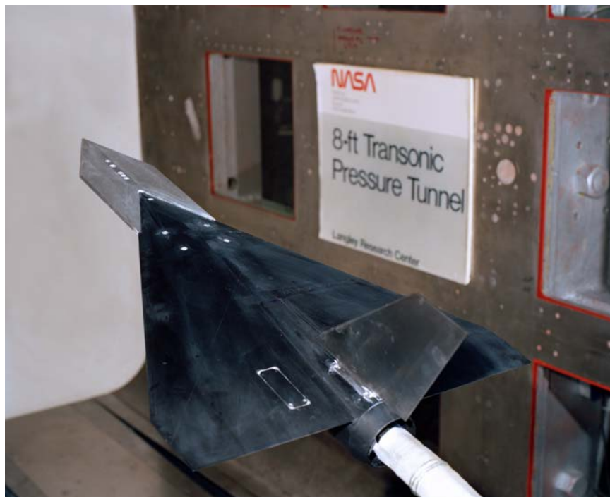
(a) Porous LEX-wing configuration with centerline tail
