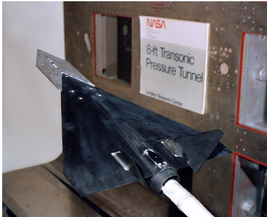
(c) Porous LEX-wing configuration with twin canted tails
