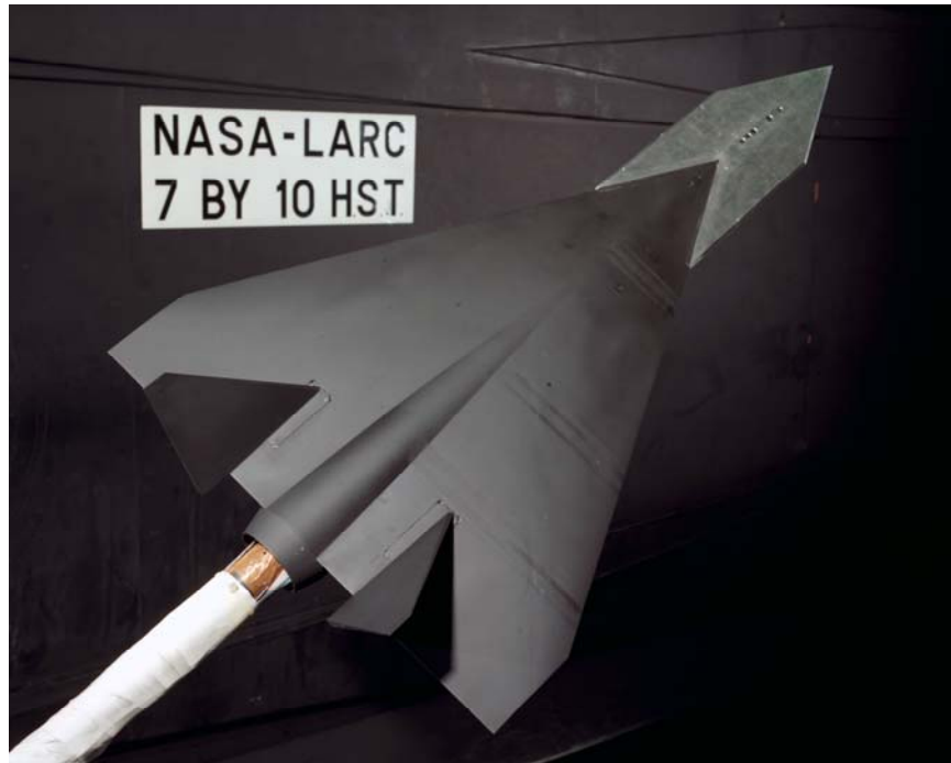
(b) 65° cropped delta wing model with porous LEX and twin canted tails
