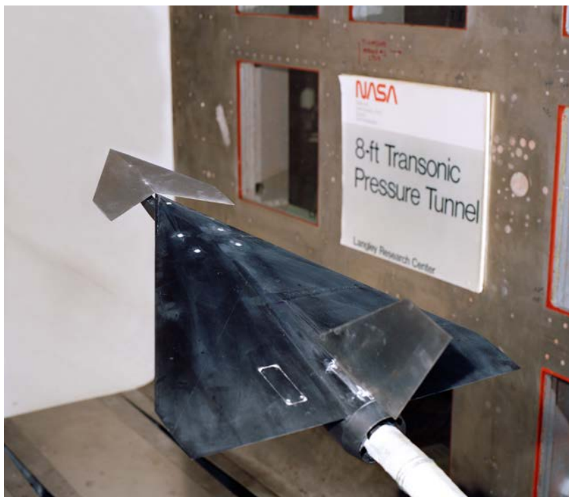
(e) Canard-wing configuration with centerline tail
