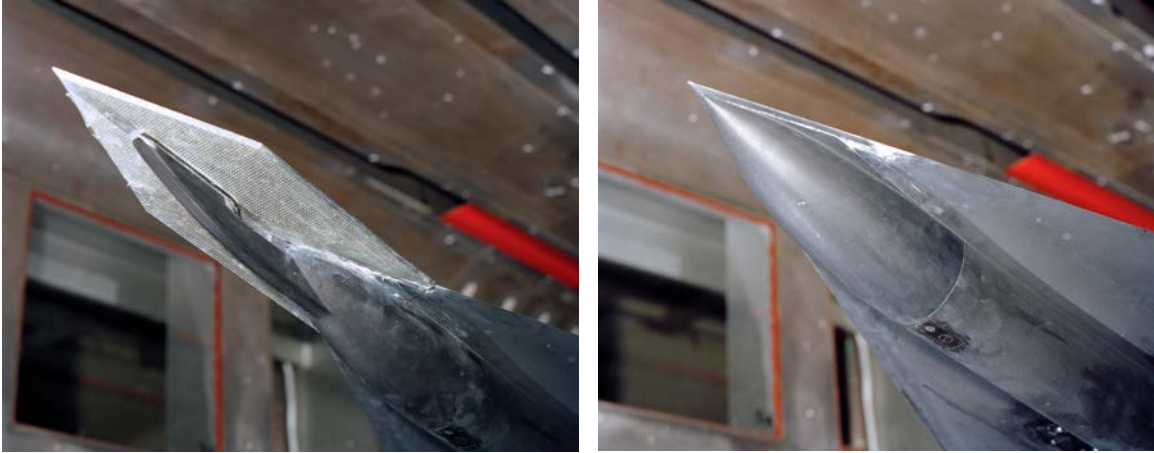
(f) Close-up photographs of LEX lower surface with gooseneck attachment to wing (left) and wing lower surface with LEX removed (right)
