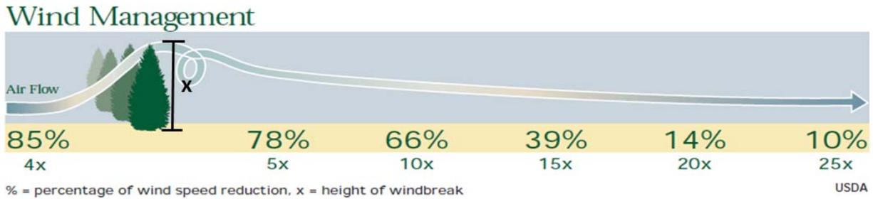
Figure 5. Wind management schematic that shows the relationship between wind speed reduction and height of windbreak. [5]
