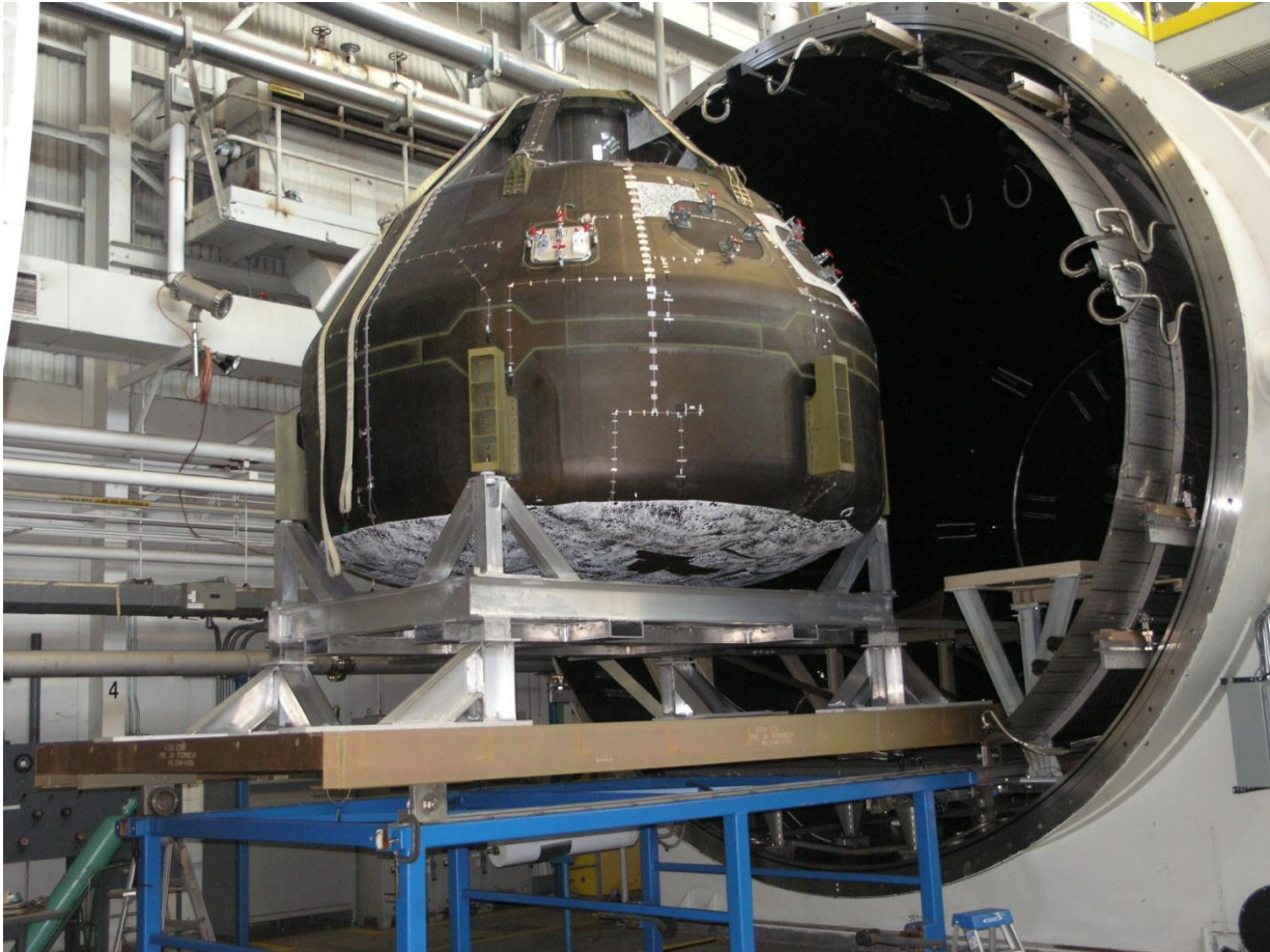
Figure 7.3-11. CCM Outside the V-20 Vacuum Chamber
