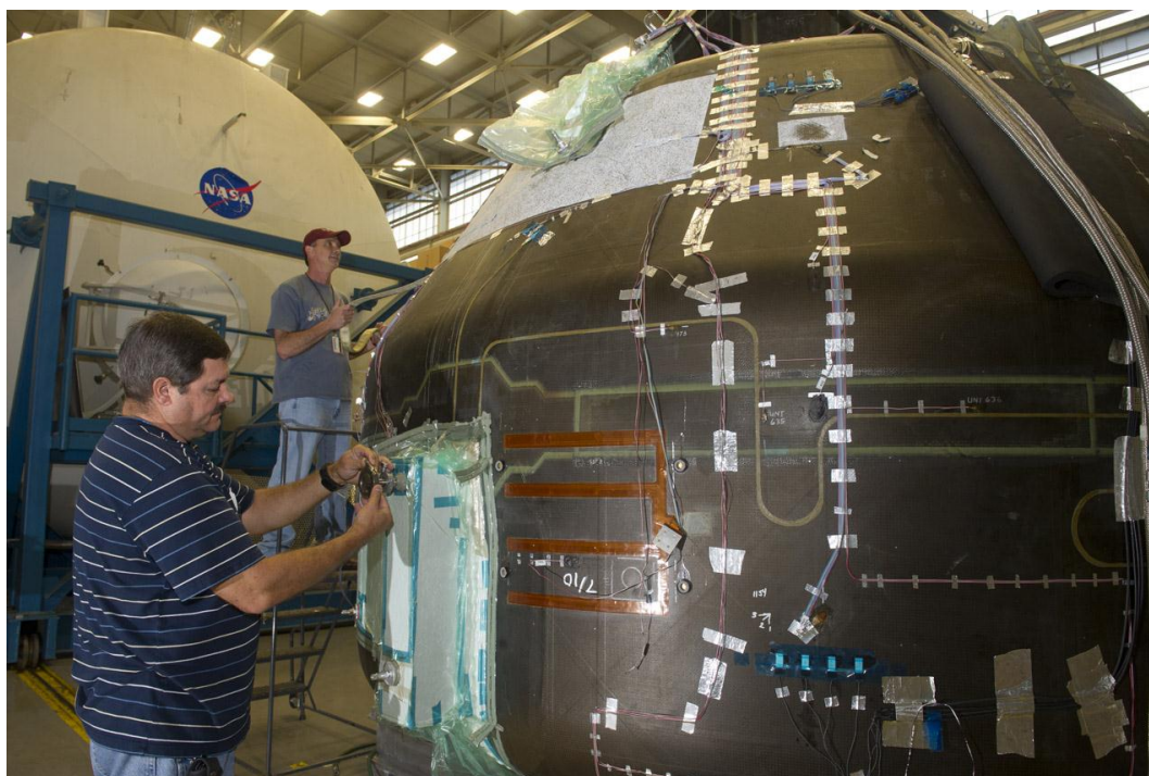
Figure 7.3-8. Vacuum Bag Installation around an SM/ALAS Fitting
