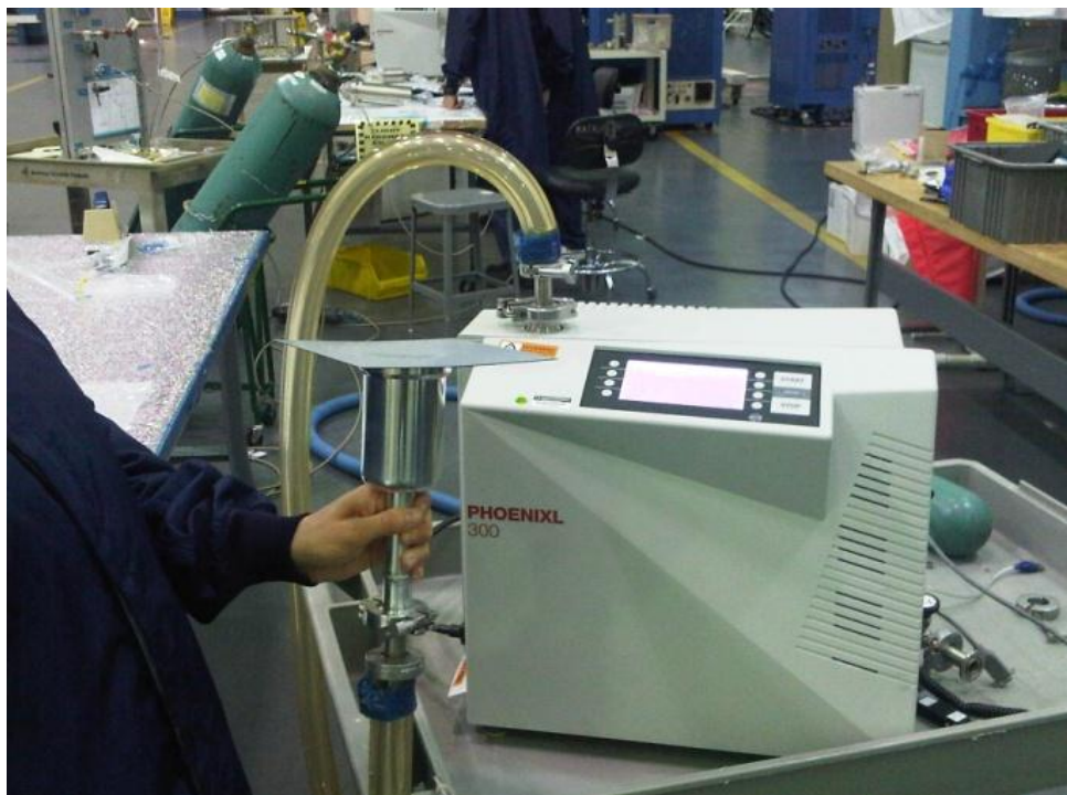
Figure 7.2-2. 7-inch × 7-inch Coupon Leak Test (helium containment bag not shown)
