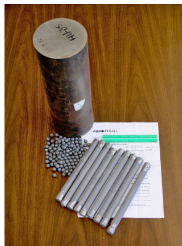
Figure 2.—60NiTi ingots and blanks produced by PM process.
