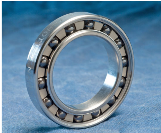
Figure 10.—Finished hybrid bearing made with 60NiTi races and \text{Si}_3\text{N}_4 bearing balls.
