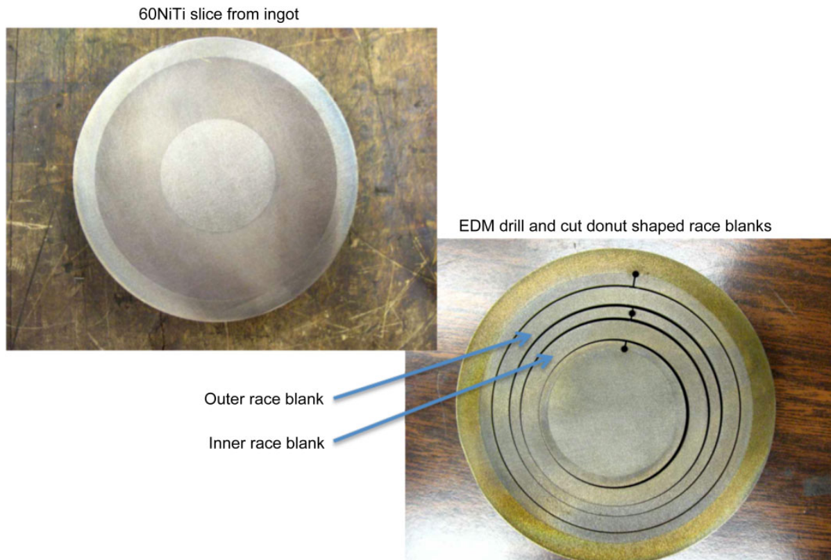
Figure 7.—60NiTi race blanks cut from ingot using EDM processes.
