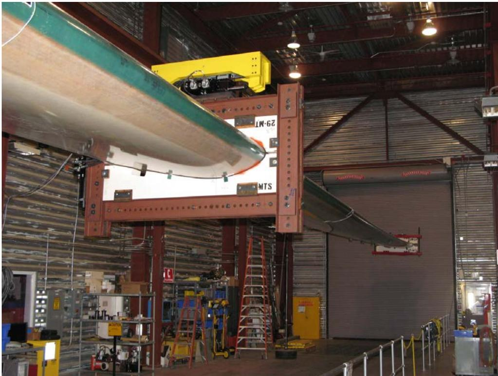
UREX configured for edge-wise fatigue test to 50m blade (PIX 20445)
