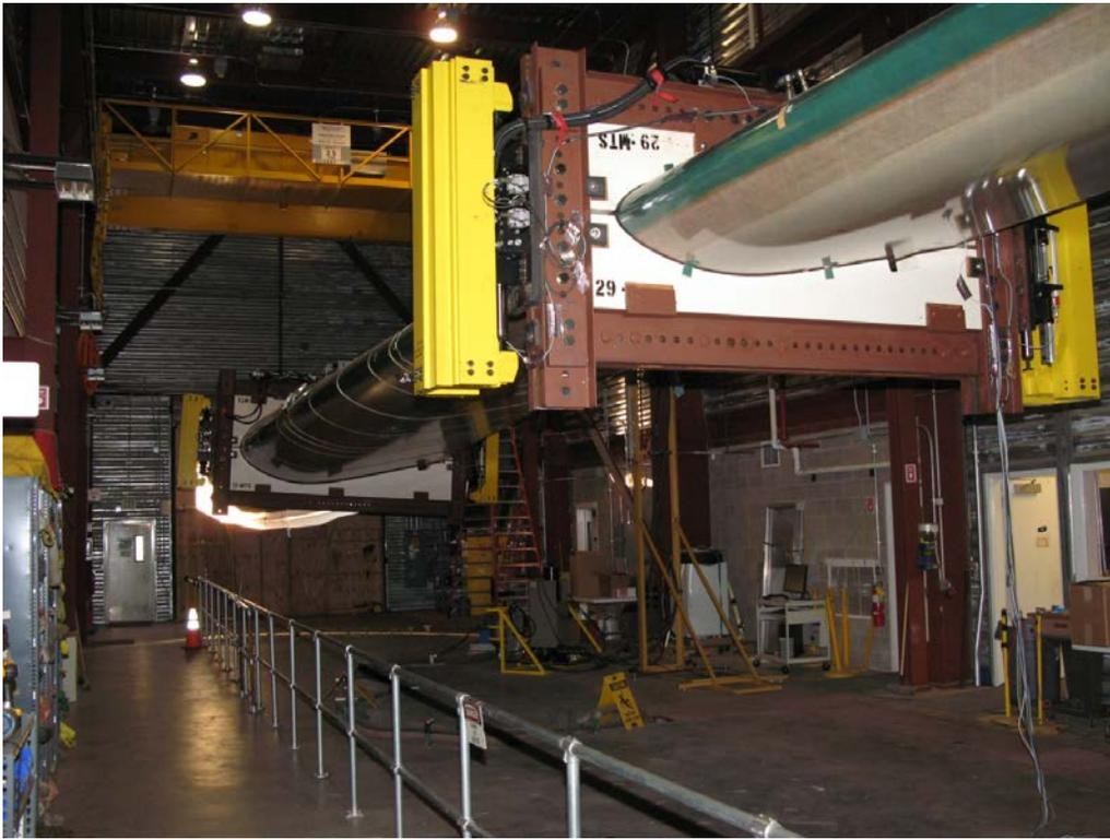
Dual-station UREX configuration for flapwise fatigue test to 50m blade (PIX 20448)
