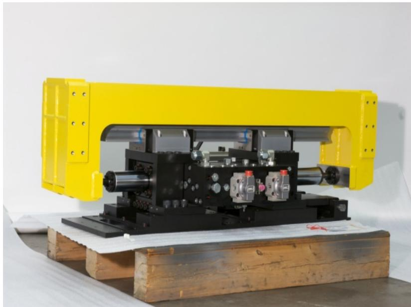
**Commercial MTS UREX resonant blade fatigue test system module developed under CRADA (PIX 17637)**
