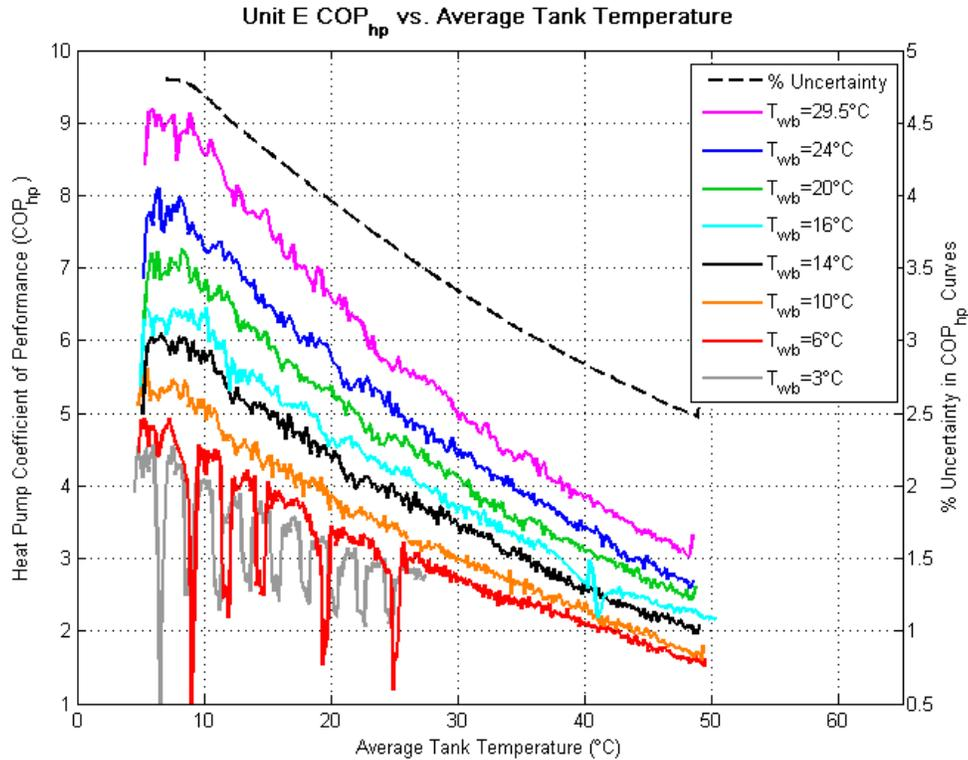
**Figure 34. COP<sub>hp</sub> traces for Unit E**
