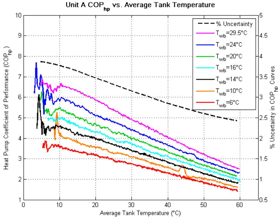
**Figure 10. COP<sub>hp</sub> traces for Unit A**
