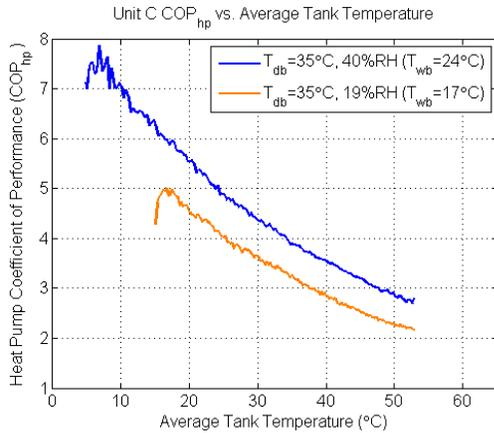
**Figure 23. Effect of humidity on COP<sub>hp</sub> for Unit C**
