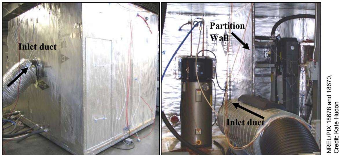
Figure 1. Test plenum during normal testing (left) and during installation (right)
