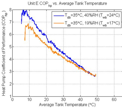
Figure 35. Effect of humidity on COP<sub>hp</sub> for Unit E
