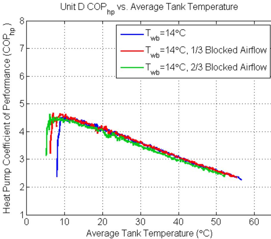
Figure 31. COP<sub>hp</sub> traces for the Unit D with reduced airflow
