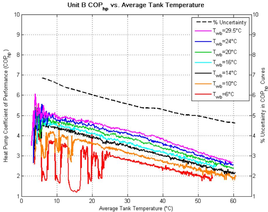
**Figure 16. COP<sub>hp</sub> traces for Unit B**
