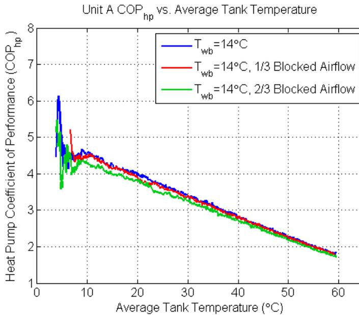
**Figure 13. Heat pump COP<sub>hp</sub> traces for Unit A HPWH with reduced airflow**
