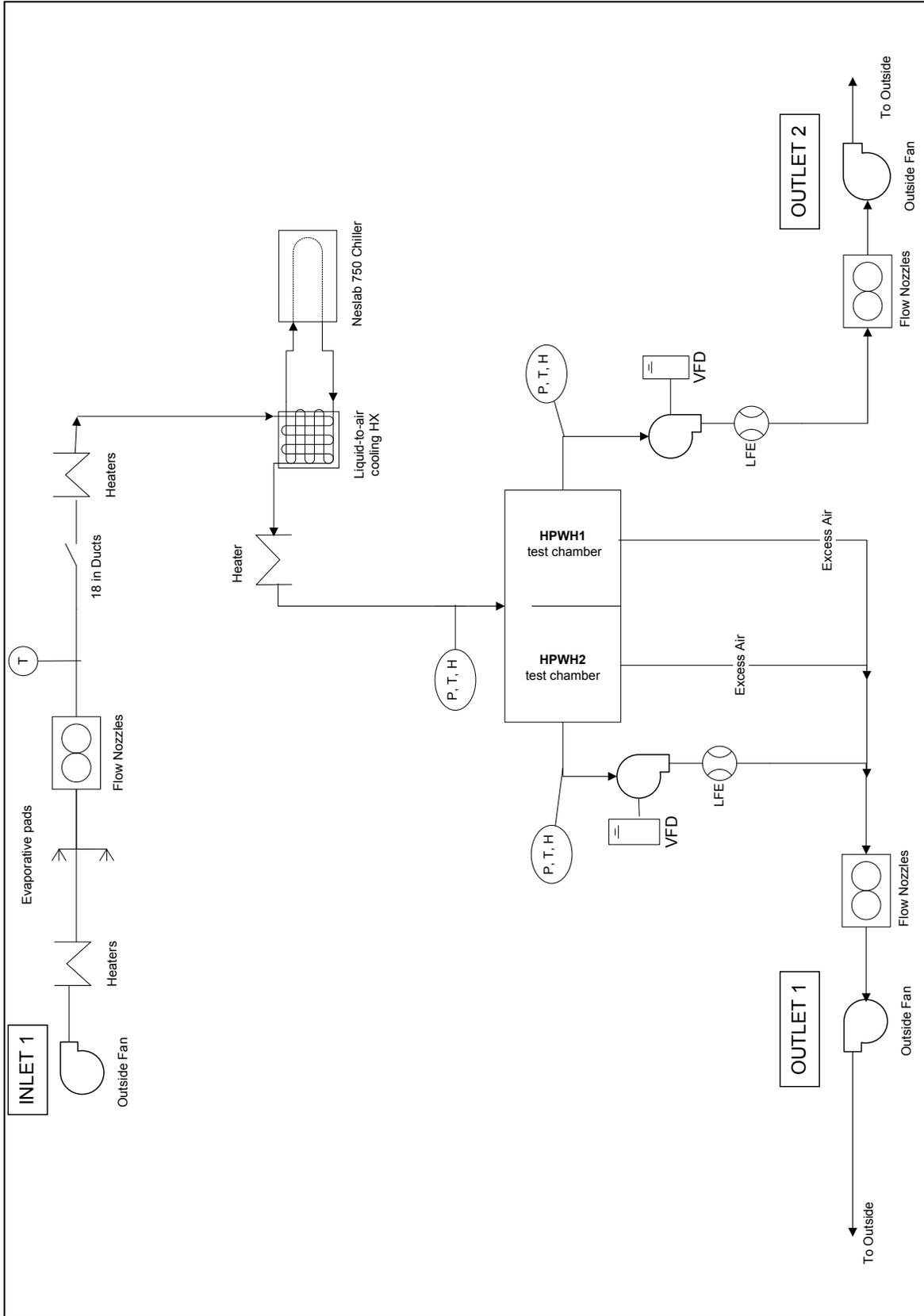
Figure 43. Air-side schematic
