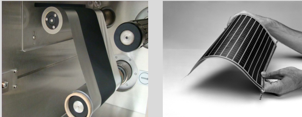
Example battery electrode (left) and thin film (right) materials. Photos from David Wood, Oak Ridge National Laboratory (L) and Warren Gretz, NREL 03541 (R)
