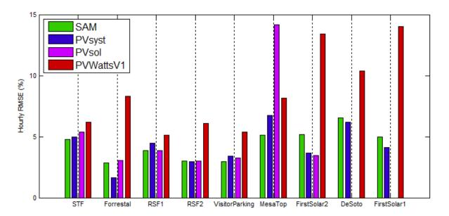
Figure 3. Normalized hourly RMSE of each tool, sorted in order of system size [1]
