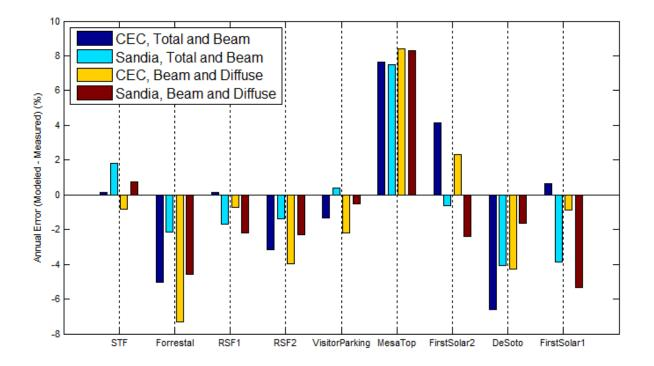
Figure 1. Annual error (modeled-measured) using different module models and irradiation inputs in SAM
