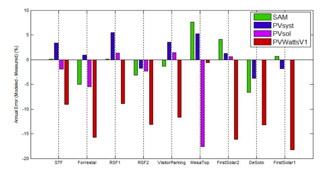
Figure 2a. Annual error (modeled-measured) using each tool, sorted in order of system size [1]
