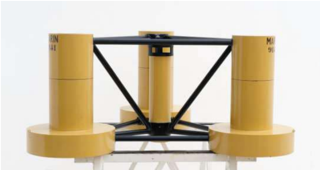
Figure 3-% As-built picture of DeepCwind semisubmersible for 1/50th scale tests
