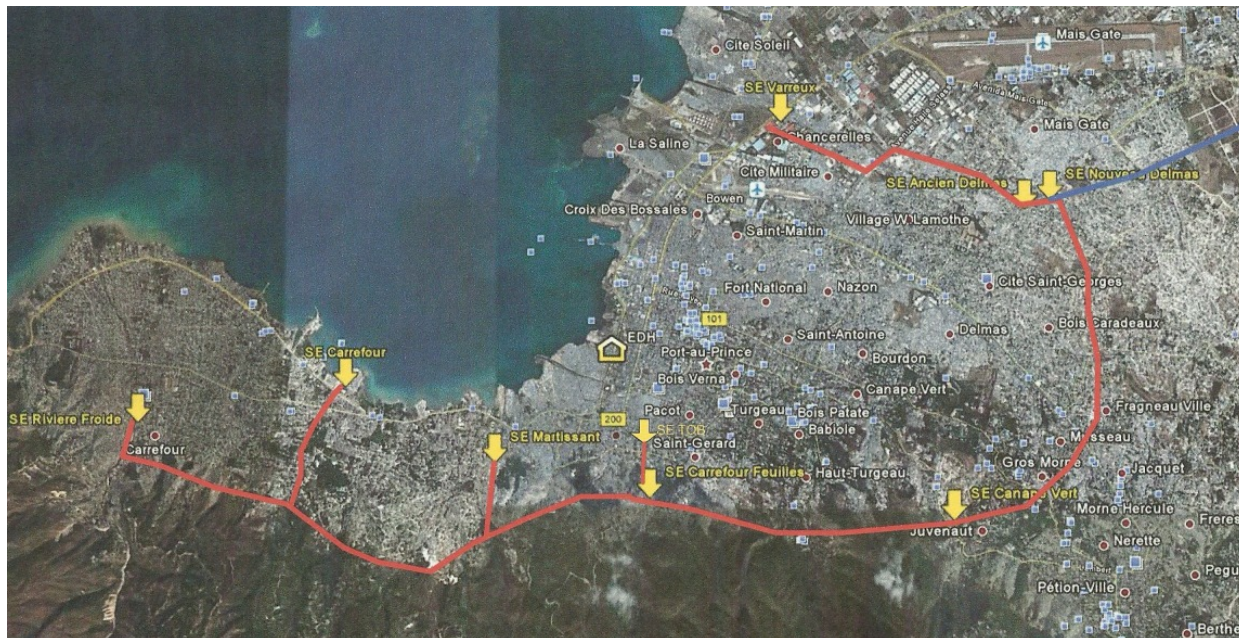
Figure 15. Transmission lines in Port-au-Prince, 2010: 69 kV (red) and 115 kV (blue)
