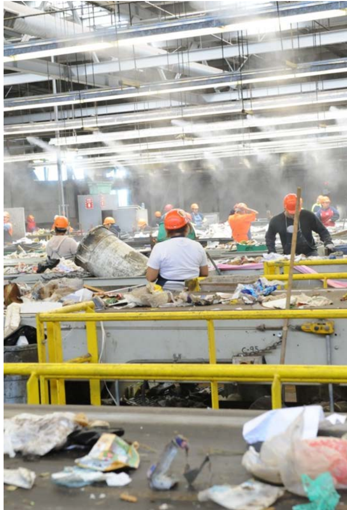
Figure 11. Typical MSW manual sorting lines (photo of the Western Placer Waste Management Authority's Materials Recovery Facility in Lincoln, California)
