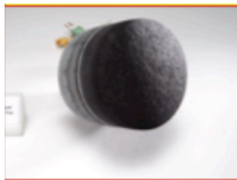
Figure 57. Post tested model at the IHF run condition - Post tested model after 75 second entry in the IHF
