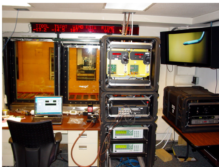
Figure 5.—NASA TWC Isokinetic System equipment in the IRT. Left, on desk, is controlling PC laptop; Center, in tall rack, are the Chilled Mirror hygrometers, the data acquisition hardware, and the IR Gas Analyzers; Right, on table, power supply that provides current for sampling probe heat.
