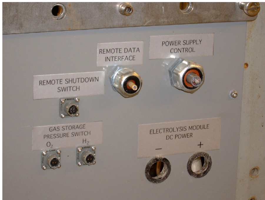
Figure 4.—Cut power and data cable interfaces.
