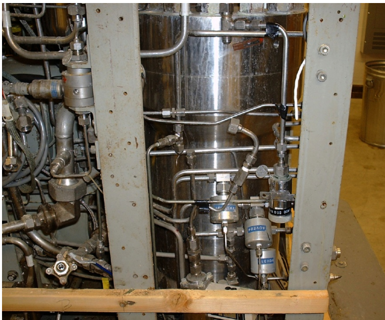
Figure 6.—Electrolyzer stack pressure vessel with disconnected fluid lines.
