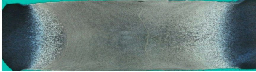
Figure 12. Transverse section of uncleaned weld. Note the fine, sharp, slightly undulating white line running from root to crown, close to the center of the weld indicating ROD.
