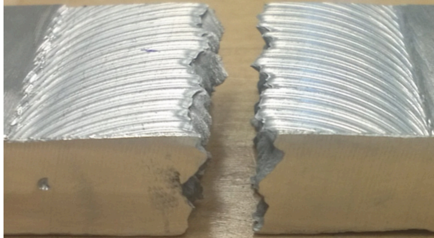
Figure 19. Fracture surface of laser cleaned weld (20 W, Adapt Laser at MSFC). Note perpendicular nonductile fracture.
