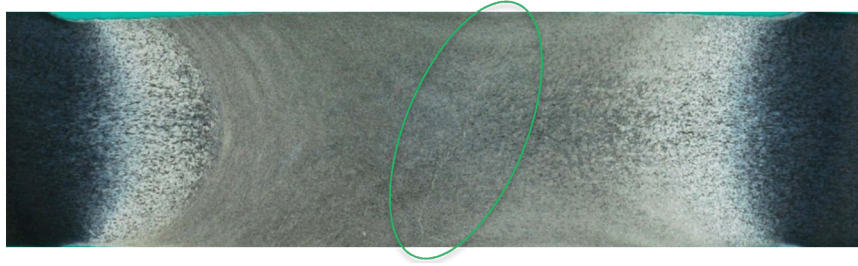
Figure 14. Transverse section of laser cleaned weld (300 W, Adapt Laser Systems). Note the fine, sharp, slightly undulating white line running from root to crown toward the center of the weld indicating ROD.
