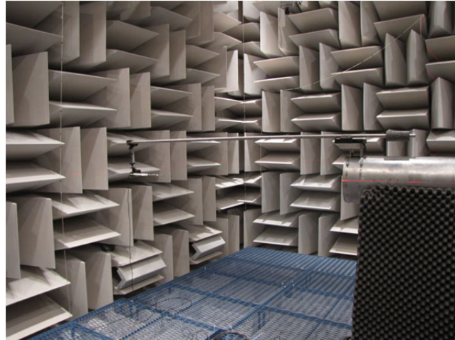
Figure 10.—Boom arm mounted to muffler for directivity survey.
