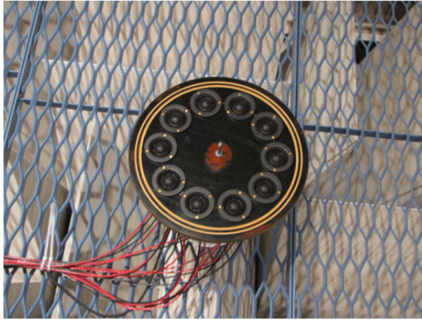
Figure 5.—Speaker plate lying on the floor of the ATL. A reference microphone is mounted in the center and extends into the hard-walled adapter.
