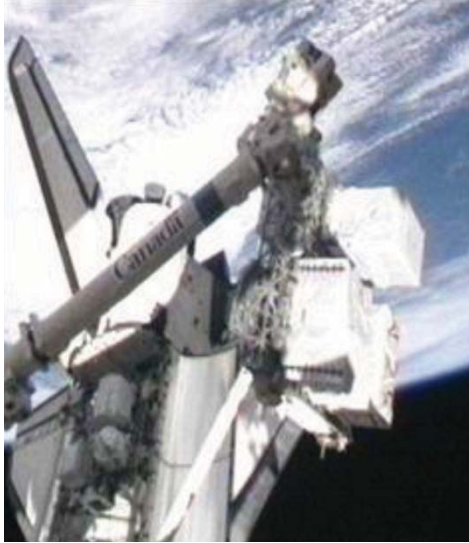
Figure 5.—Relocation of ELC1 from Shuttle cargo bay to ISS.
