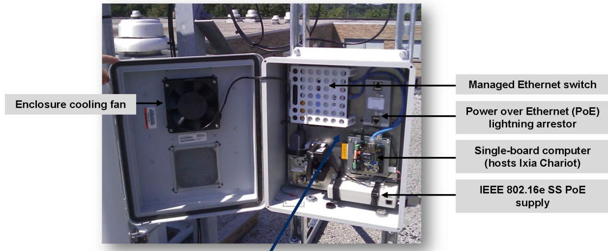
Figure 38.—Internal electronics of subscriber station enclosure.
