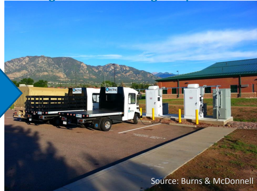
5x 60-kW Bi-directional Stations Integrated with Microgrid Operations
