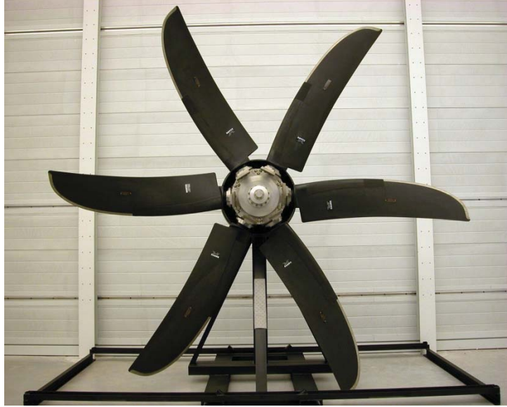
Figure 1.—Surrogate blade provided by the FAA.
