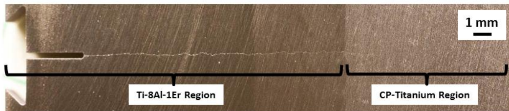
(c) Ti-8Al-1Er to CP-Titanium Gradient Specimen
