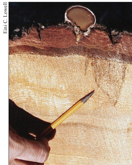
Figure 3—Pouch fungus conk on a cross section of 2-year-dead Douglas-fir log and associated sap rot.
