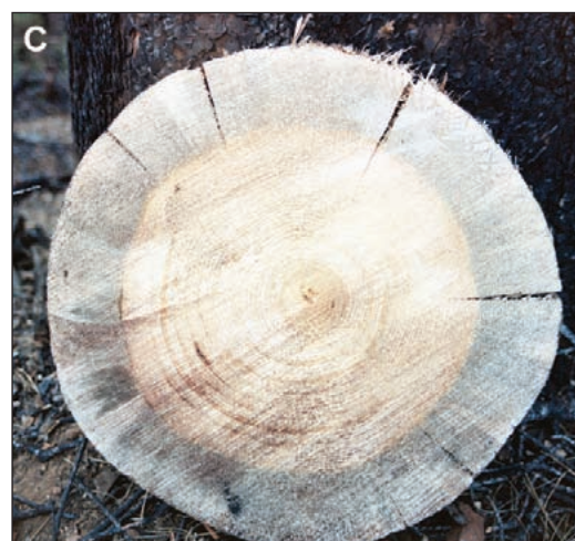
Figure 6—Weather checking in (A) standing trees (beetle-killed lodgepole pine), (B) logs (beetle-killed lutz spruce), and (C) cross section (fire-killed ponderosa pine).
