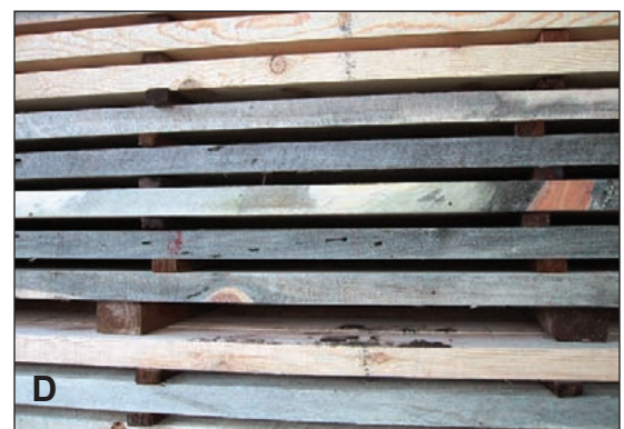
Figure 10—Blue stain in fire-killed ponderosa pine (A) tree, 3 months following fire, (B) end of a log, (C) sawn cant, and (D) side of lumber stack.
