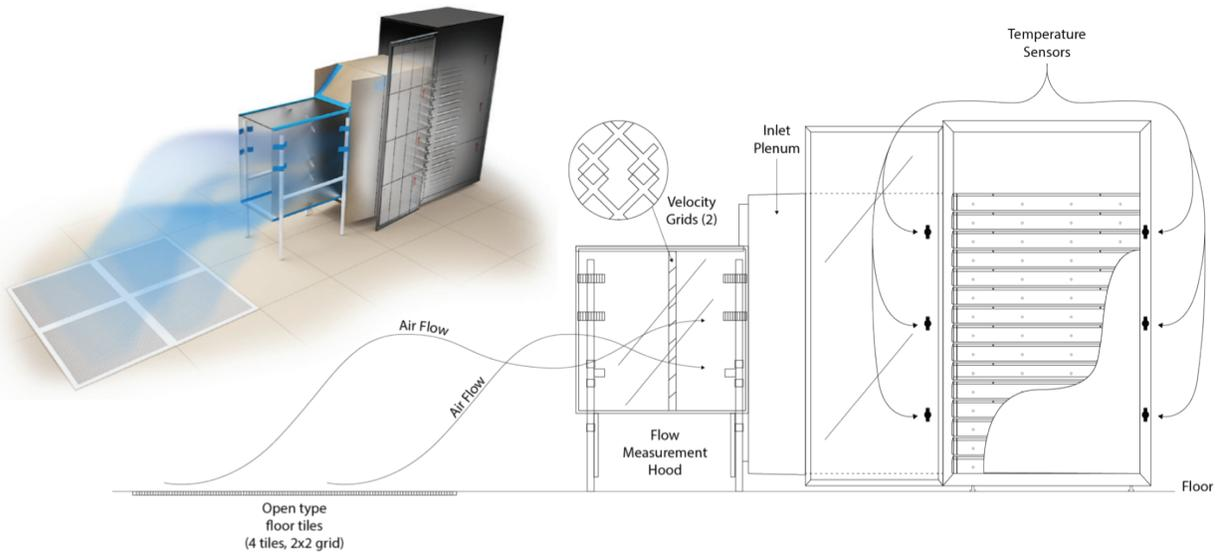
**Figure 6. Test setup.**
