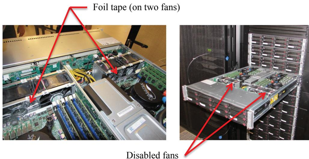
**Figure 9. Server fan configuration during aggressive second retrofit attempt.**
