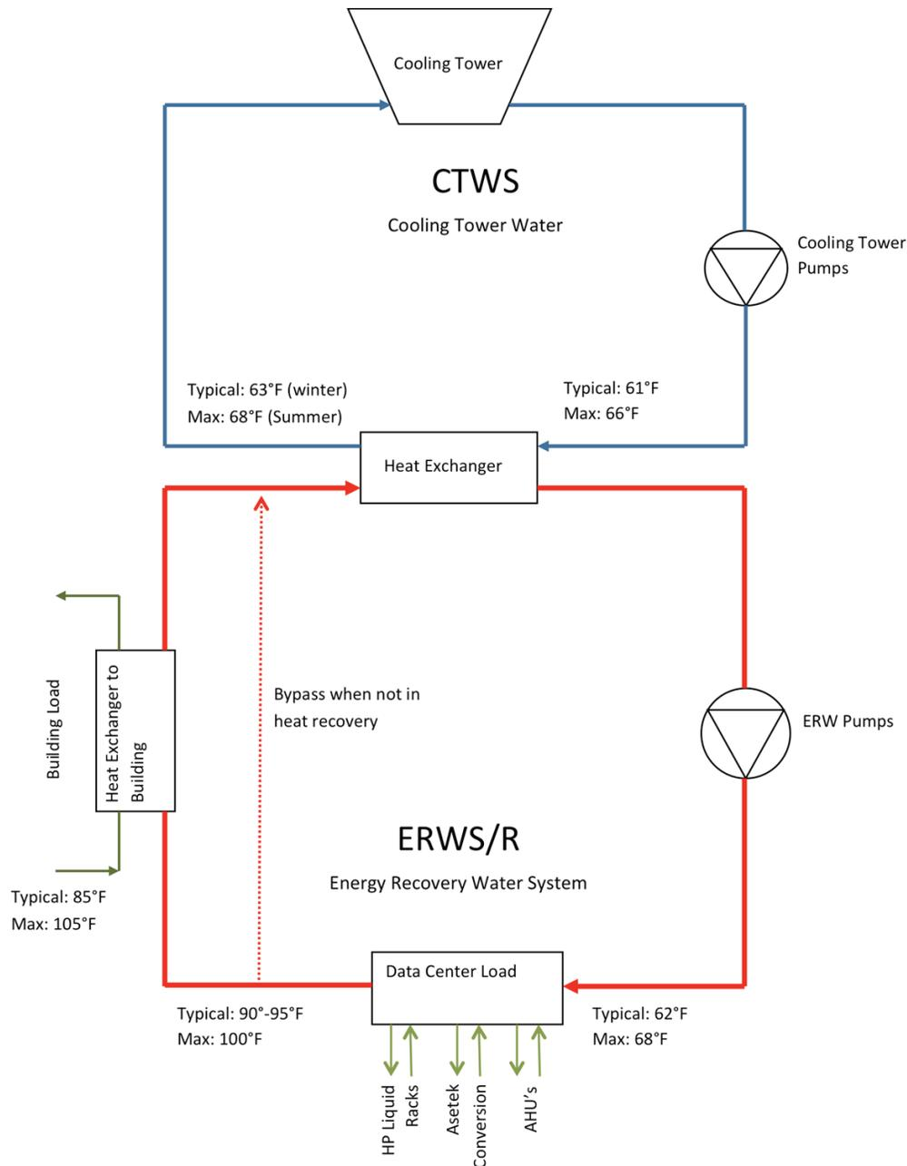
**Figure 7. Building-level system diagram.**
