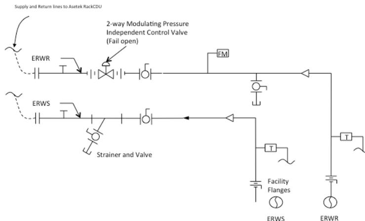
**Figure 8. Line drawing of facility pipe additions to support Asetek RackCDU.**
