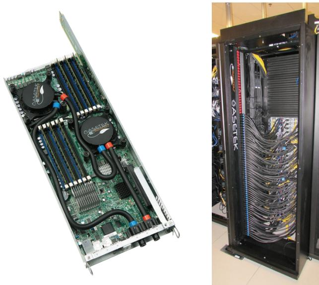
**Figure 1. Asetek pump/cold plate units and RackCDU.**
