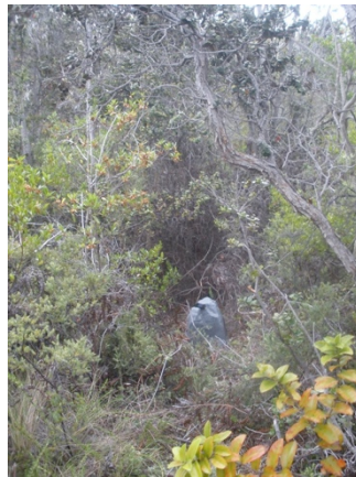
Figure 3. Photograph showing the sensor and bucket at array AIND covered with a fake rock and placed in an ideal location in the shrubbery to reduce wind noise (element 04).
