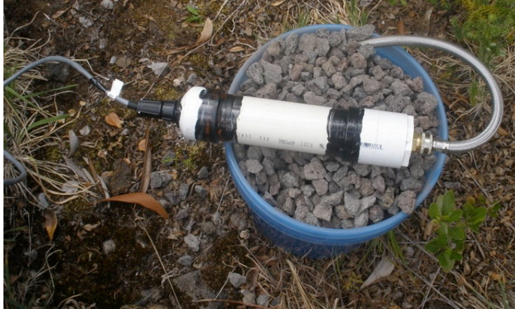
Figure 2. Photograph showing the pressure sensor enclosed in piping and resting on top of the bucket containing washed gravel and a buried screened inlet.
